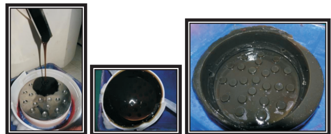
Fig. 8: Steel template was duplicated in reversible hydrocolloid material
