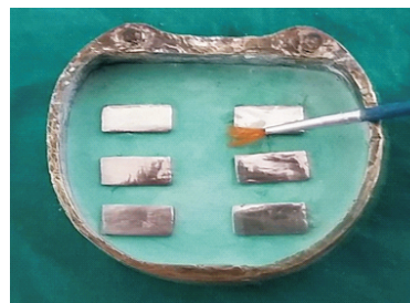
Fig-1.Master die invested in Type III dental stone
