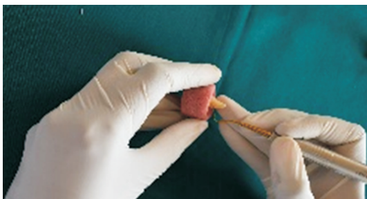
Figure 2: Application of self-etch adhesive and composite to each half of the sectioned tooth in increments.
