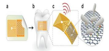
Biotransferrable graphene wireless nanosensor. (a) Graphene is printed onto bioresorbable silk and contacts are formed containing a wireless coil. (b) Biotransfer of the nanosensing architecture onto the surface of a tooth. (c) Magnified schematic of the sensing element, illustrating wireless readout. (d) Binding of pathogenic bacteria by peptides selfassembled on the graphene nanotransducer.
