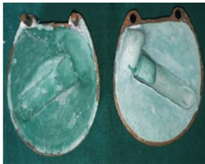
Figure 10: Dewaxing of wax pattern.
