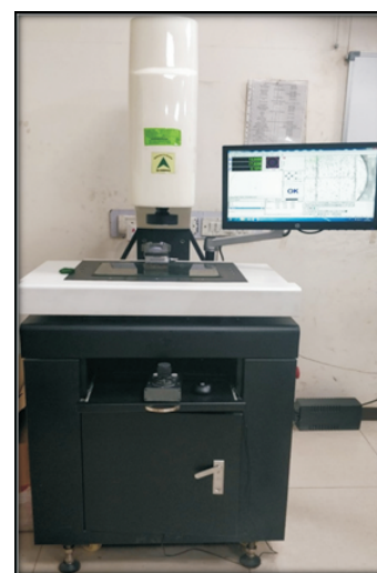
Figure 6: Vision measurement machine measuring the master model dimensions
