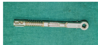
Fig.-3 Torque ratchet with calibration
